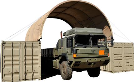
The Workshop Shelter is a rapidly redeployable shelter which can be mounted on ISO shipping containers by means of special beams with connections into the ISO locks.
